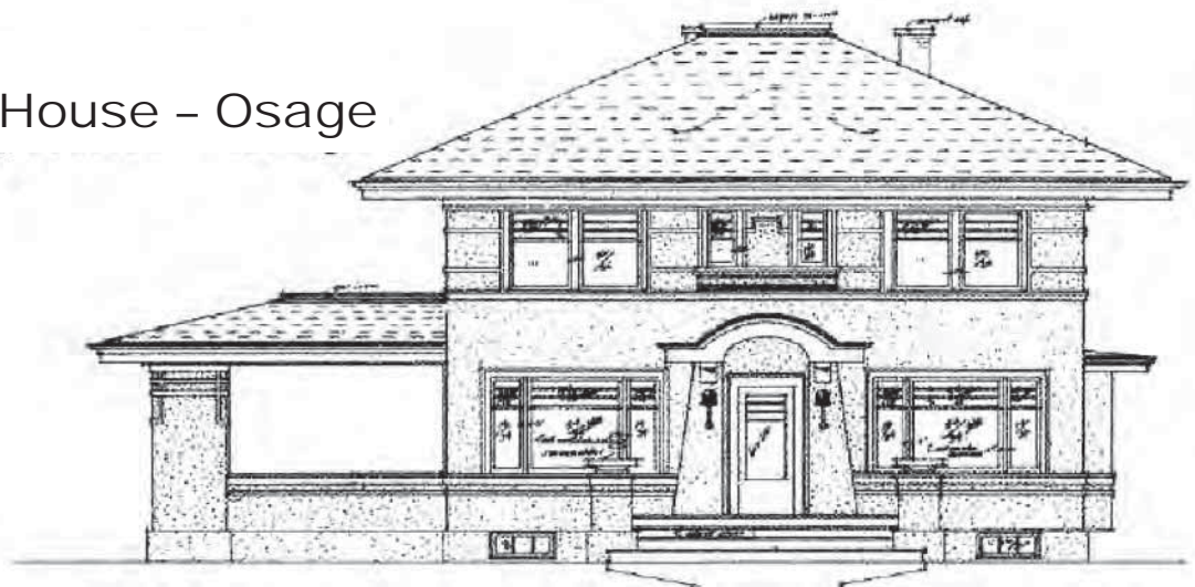
Figure 34 The Husting residence, an elongated Foursquare type house in Osage, Iowa, some 40 miles northwest of Waterloo, was planned in 1916 with a flanged-arch front entrance porch roof, supported by two battered columns. A hint of an eyebrow dormer on the roof above – erased on the plans and discarded by Burr and his client – is still visible in this image. Taken from Nash, "Howard Burr: Master of the Prairie School" (1991).
