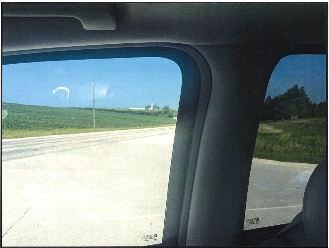
W 51 looking Westbound onto IA 56 toward an oncoming truck hidden behind the car post
