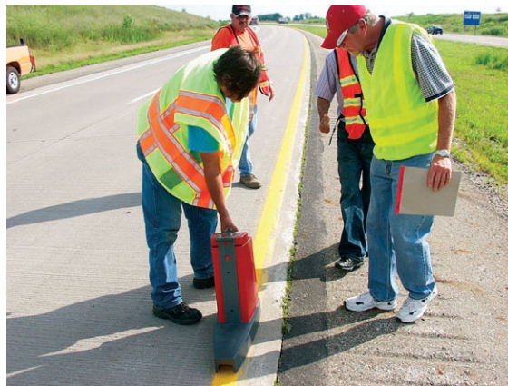
Iowa DOT crews learn how to use reflectometer equipment to ensure proper paint application and maintenance. New materials and quality-controlled application can help provide drivers with more visible and resilient pavement markings.
