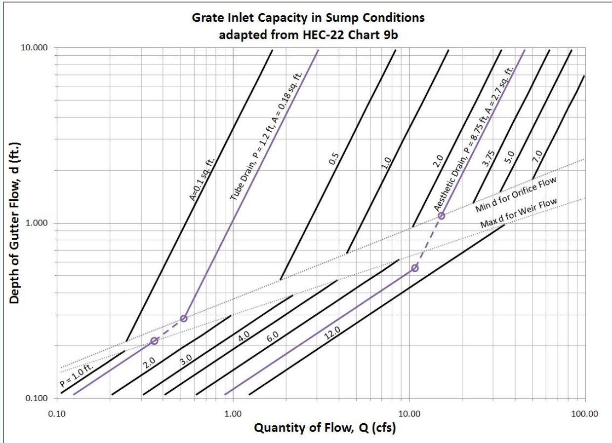
Figure 5: Grate Inlet Capacity in Sump Conditions
