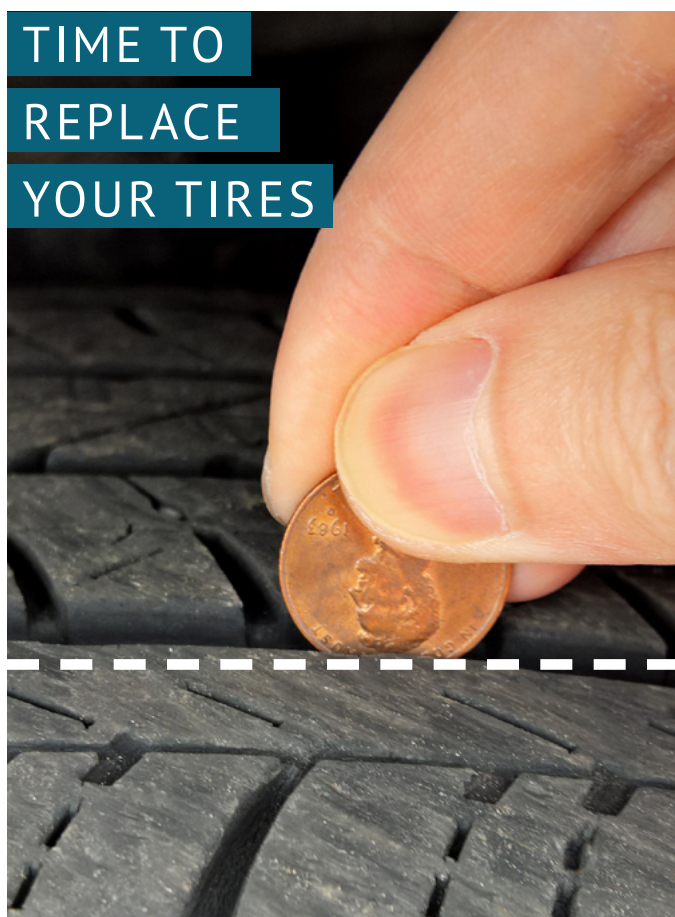
Figure 3.1: Check your tire tread with a penny
