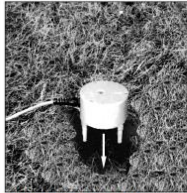
Figure 3.4 Installing the Standard Transducer using the Ground Spikes.
