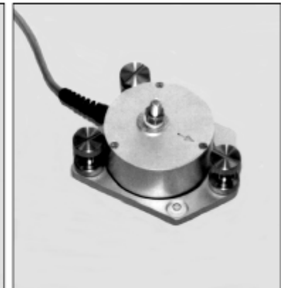
Figure 3.12 Bolting the Standard Transducer to a Surface using the Leveling Plate.
