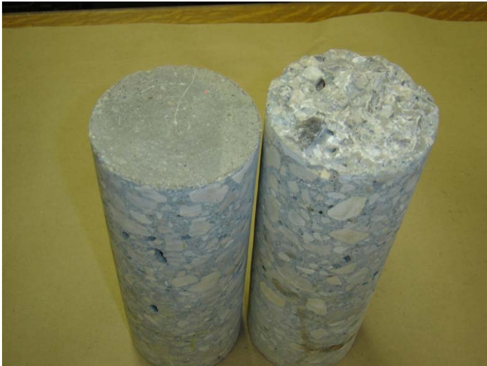
Figure 7 Core bottom showing difference between on target versus granular subbase.
