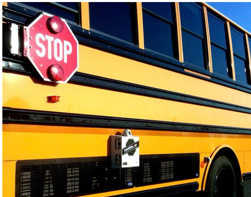
Figure 7. Stop-arm violation camera (Gatekeeper Systems Inc.)
