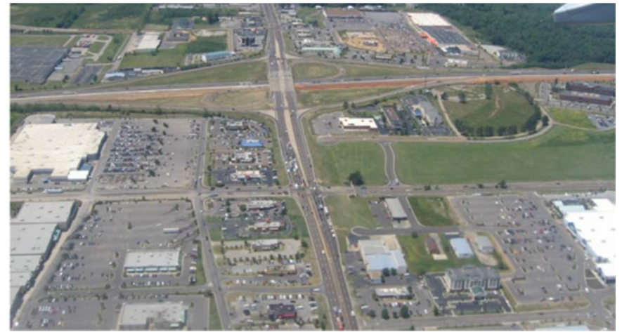
Figure 22: Interchange area with limited crossroad access, but with good local street circulation supporting retail developments (Mississippi)
