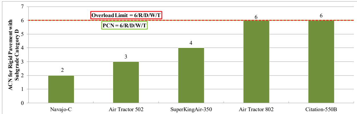
Figure 2. ACN–PCN comparison for Runway 16-34.
