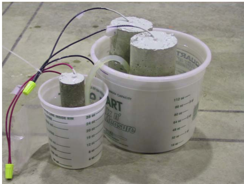
(b) – Typical as-constructed Rapid Macrocell ACT
