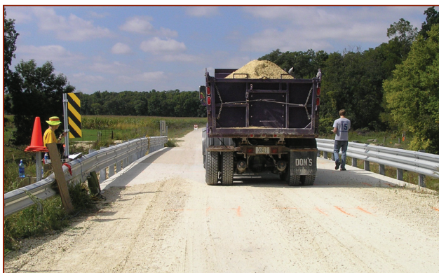
Load testing the bridge was part of the structural performance evaluation
