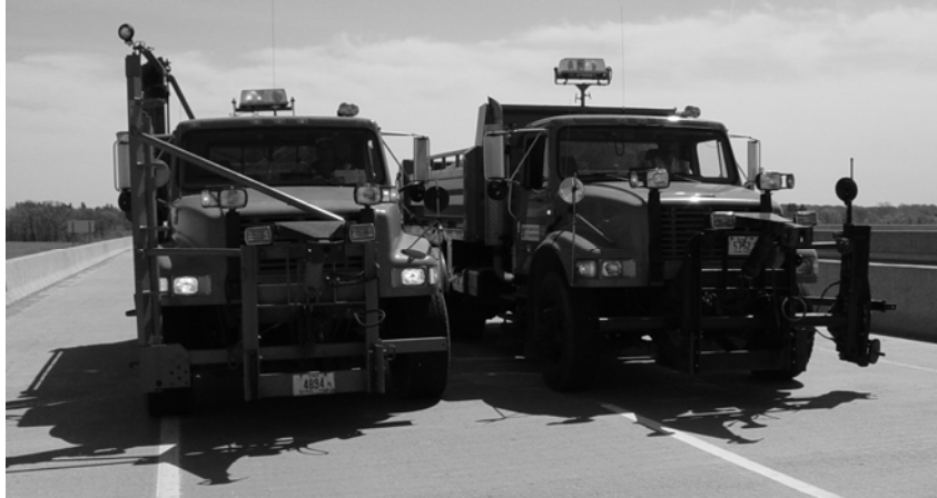
FIGURE 9. Test trucks used for load rating test prior to passage of superload vehicle.
