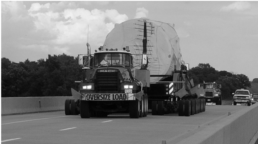
FIGURE 12. Superload crossing the prestressed girder bridge during load rating test.
