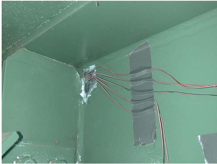
a. Typical web gap gradient instrumentation (bridge 5075.5R080 shown).
