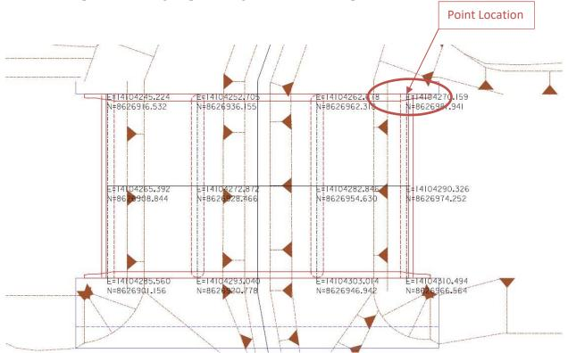
Place the cell 'Brg\_Coor'. Edit the cell appropriately and move the coordinate text elements from the bridge diagram into the table.
