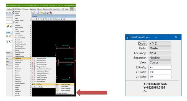
The Label Coordinates tool allows a change in the accuracy of coordinates and the X and Y prefixes can be changed to E and N respectively. The coordinates should be placed on the brgTextNormal level with the appropriate attributes. Note that the Label Coordinates tool uses the active text settings.
