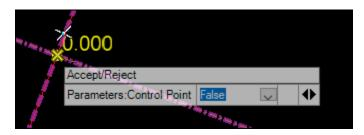
Reposition the point, if needed, by using the select tool to select the point. Hover over the point to get the 'Move' command. Move the point to a new location.
