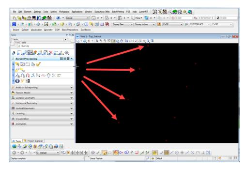
Now that the replotted points are in a blank file that has the correct projection assigned to it for this project, the project files can be attached (survey, road design, preliminary bridge) as references to help validate that the eFile is correct.
