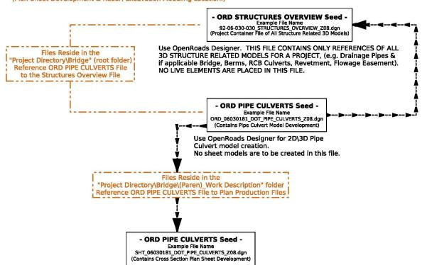
Use OpenRoads Designer, reference in 2D\3D design model and use ORD "Placed Named Boundary Civil Cross Section" tool - "Civil Cross Section 2 Points" to create drawing models referenced to sheet models.
