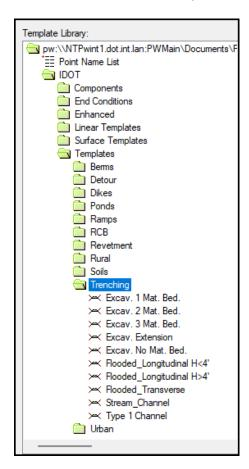
The list of available linear templates for RCB Culvert Excavation (Trenching) modeling in ORD is shown below.
