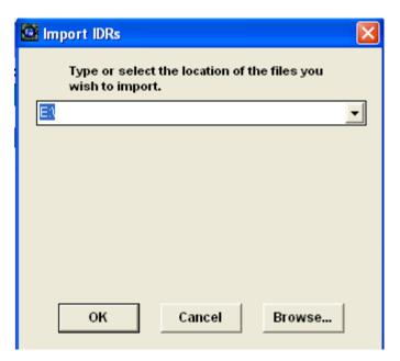
The program will not ask for the name of the file, just the location. The files created by the inspector are automatically named and have the extension of .EBL. When the FieldManager program imports a file from FieldBook, it looks for any file in the specified location with an extension of .EBL and imports it.
