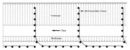
EC-201 showing silt fence installation in shallow or no ditch situation.
