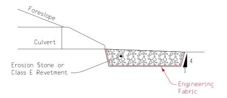
Detail of splash basin at a culvert.
