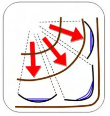
Above illustrations show placement of silt fence along contours of a slope. (The brown lines represent contour lines.)
