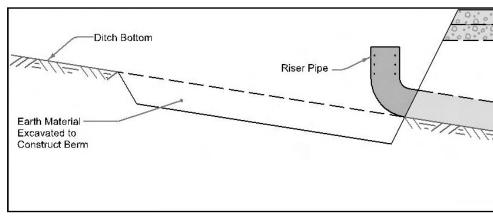
Profile of a temporary sediment control basin.
