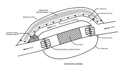
EW-402 provides for different methods the contractor may use to divert flow of a stream. As shown above, a diversion channel is one of the methods. Using a pipe or hose is another method to divert the flow.
