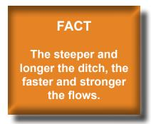
Erosion may create gullies in the ditch making it difficult to install silt fence ditch checks. The ditch may require re-grading prior to installing the ditch checks.
