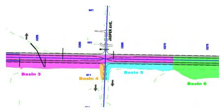
Plan sheet showing color coded drainage basins and discharge points
