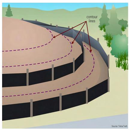
This illustration shows multiple rows of silt fence installed <u>along</u> the contour lines.
