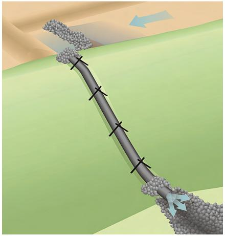
This illustration shows a temporary slope drain. Though not commonly used in lowa, other states have used this type of control to convey water through a pipe over a disturbed slope.
