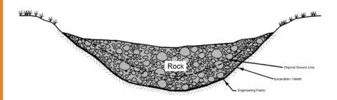
Rock Check Dam detail for temporary applications.
