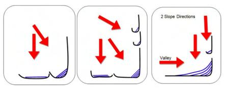
These are examples of correct silt fence placement where a single section of silt fence is broken up into multiple sections with J-hooks. Multiple sections provide multiple storage areas for water to accumulate, thus reducing the chance of a blow-out.
