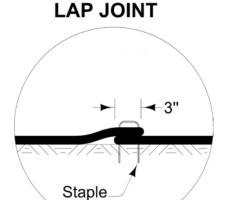
When a new section is added, it should be placed 3 inches over the previous section of fabric and stapled in place.
