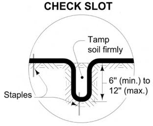
Check slots should be used in ditches with slopes of more than 4%.
