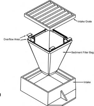
This type of inlet protection uses a sediment filter bag Inlet protection will serve to slow the water down and may result in creating some ponding upstream of the inlet. Because of this, there is potential for inlet protection to create flooding hazards, and these areas should be monitored closely during rain events.
