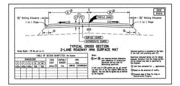
Spread rates for hot mix asphalt are normally found by using the contract quantity of mix as a basis. If the contract quantity is not sufficient to construct the required thickness, notify your supervisor as soon as possible. If necessary, the Construction Residency can contact the District Office to obtain spread rate adjustments required to obtain the design thickness.
