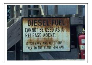
Do not allow the use of diesel fuel, kerosene or distillates for cleaning truck boxes or other equipment that comes into contact with the mix. If treated with distillates, trucks must drain for a minimum of 5 hours prior to being used to haul mix. Approved release agents are found in Materials *IM* 491.15.
