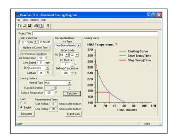
Wind velocity, air temperature, and cloud cover are additional factors that affect the cooling rate of HMA. *PaveCool* is a software program, developed by the Minnesota Department of Transportation and Minnesota Asphalt Paving Association, used to determine approximate cooling rates for hot mix asphalt pavement under various conditions. The program uses numerous variables to graph cooling curves and provide a resulting "time available for compaction" following mix laydown.
