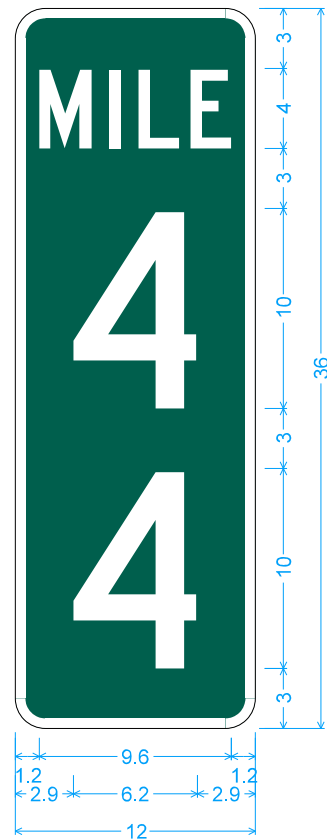
D10-2A; 1.50" Radius, 0.50" Border, White on Green; [MILE] C 2K; [4] C 2K; [4] C 2K;
