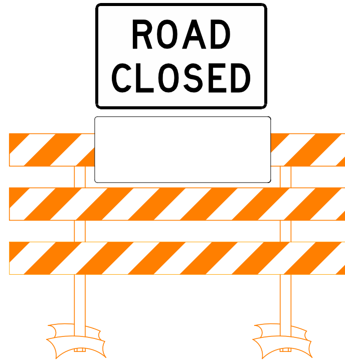
Sign Placement with Supplemental Sign
