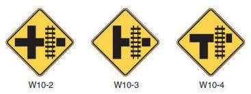
Figure 4: W10 series warning signs for grade crossing (2009 MUTCD).
