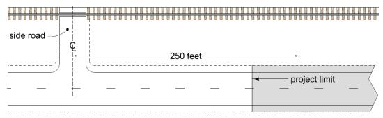
Figure 1: Project limit within 250 feet of side road centerline.
