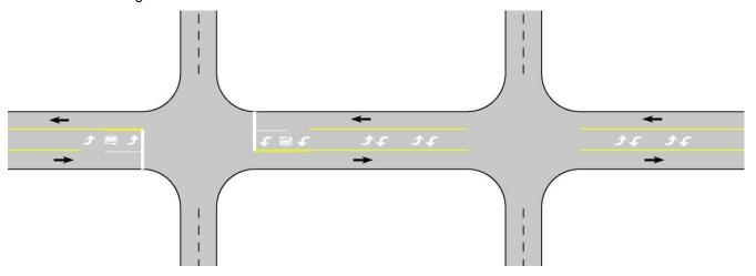
Figure 5: Continuous two-way left-turn lane.
