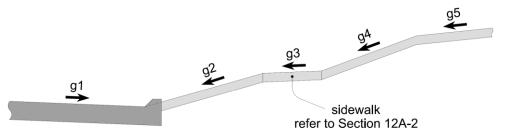
Type B, C, and D accesses: g2, g4, and g5 should not exceed 14% and should be as flat as possible for Type B high volume traffic accesses.
