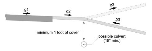
Type B, C, and D accesses: g3 should not exceed 14% and should be as flat as possible for Type B high volume traffic accesses.
