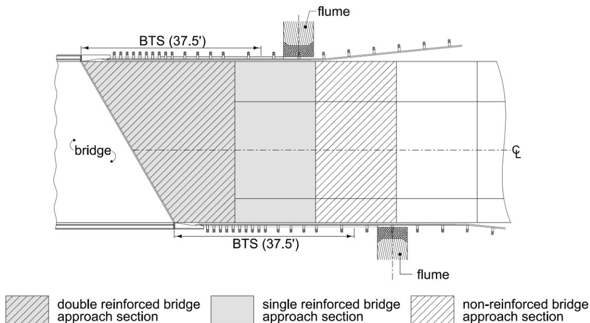
**Figure 2:** Placement of flumes.
