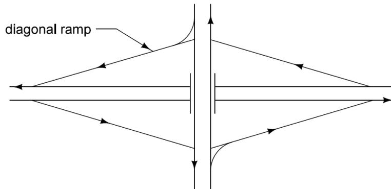
**Figure 2:** Diagonal ramp at a diamond interchange.
