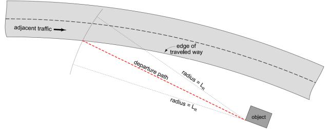
Figure 6: Departure path on the inside of a curve.
