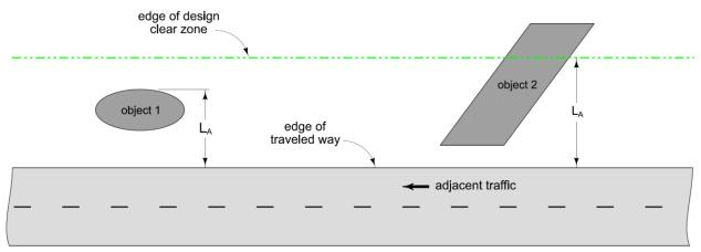
Figure 2: Comparison of L<sub>A</sub> distances for different objects.
