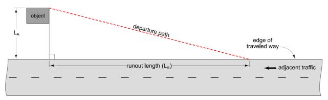
Figure 3: Establishing the departure path.
