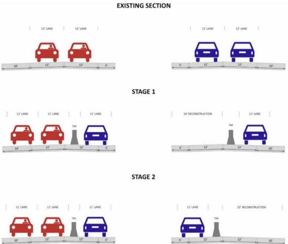
Figure 1: Contraflow concept for four lane divided highway.
