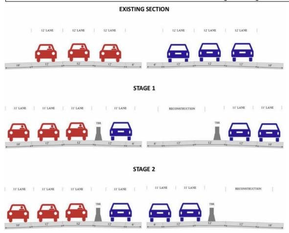
Figure 2: Contraflow concept for four lane divided highway.
