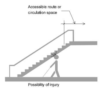
Figure 12A-3.03: Shielding for Vertical Clearance Obstacles
