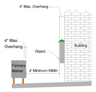
Figure 12A-3.04: Horizontal Clearance
