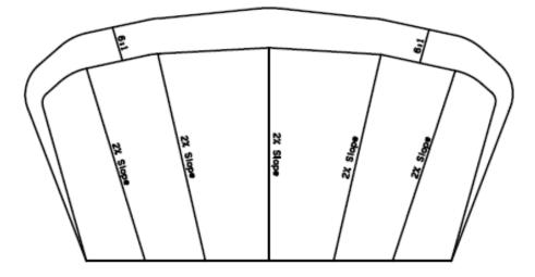
Figure 3: Example Drainable Borrow Plan.
