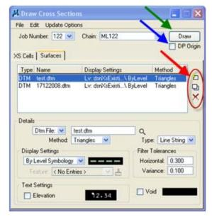
Details – select between DTM File and Tin file, as shown at the right. DTM file: This option will be used when generating cross sections with Corridor Modeler for both the existing ground and proposed surface created through Roadway Designer.
