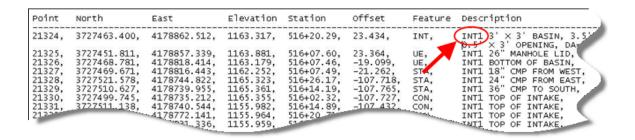
10.) The feature code INB should be used when surveying bee hive intakes. The location of the INB shot should be at the center of the intake and at the surface flow elevation. With the exception of the IN feature, all other shots required shots are the same as for a standard intake.
