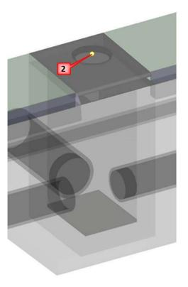
4.) It is important for the designers to know if the MH has lift rings inside that total more than 16". It is required to identify how many lifts there are and the thickness of each lift. This information should be placed in the UE for the manhole lid description. A photo of the inside of the manhole that shows the lift(s) while holding a ruler vertically against it would also be beneficial.
