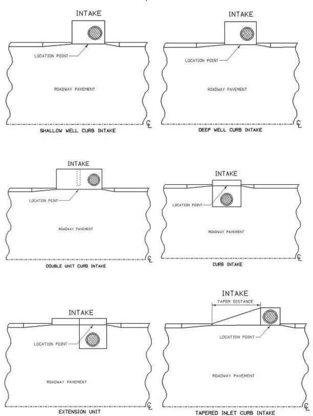
3.) Shot number 2 is taken on the center of the manhole cover, if present. This shot should have the feature code of UE (Utility Elevation) and the description should be the size of the lid (26" MANHOLE). The UE feature is used instead of MH (Manhole) because the drawing becomes too cluttered in MicroStation if the intake and manhole cell are both drawn.
