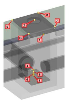
2.) The first shot, with a feature code of IN, determines the location of the intake. A cell representing the intake will be drawn at this location in the MicroStation file. The description for this point should contain the BASIN SIZE, COVER SIZE, CONDITION (including amount of silt), LENGTH OF OPENING and DRAINAGE AREA.
