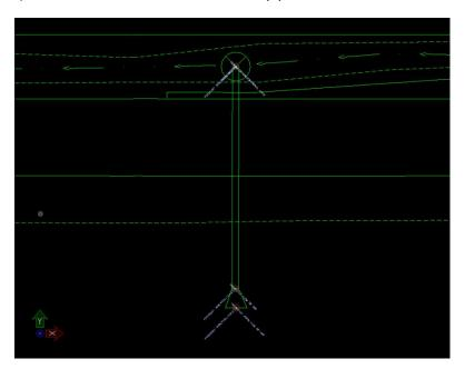
9.) The first item entered in the description field for each intake shot intake is an identifier, as shown below. The easiest way to name the intake identifiers is to start with the name of INT1 for first intake surveyed. The identifier number for each intake surveyed thereafter will sequentially increase, e.g., INT2, INT3, INT4. This identifier will be used by the customer to group all shots together that are associated with each drainage structure.
