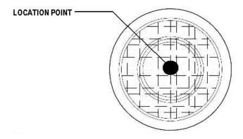
11.) Manholes that are not related to an intake should be shot with the feature MH. All other features related to the manhole should be collected in the same manner as for the standard intake.
