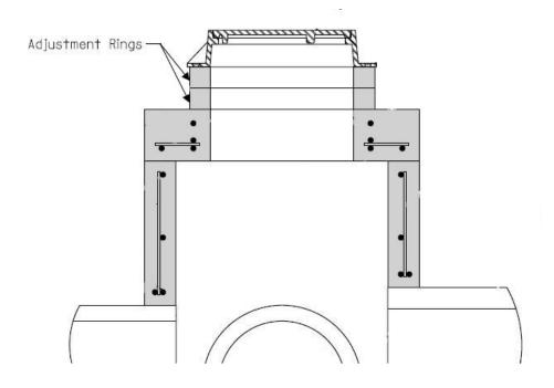
5.) Point 3 is the bottom of the well shot and should have feature code UE. This shot should be at the same XY location as the point 2, the center of the manhole cover. The description for this point should be BOTTOM OF BASIN.
