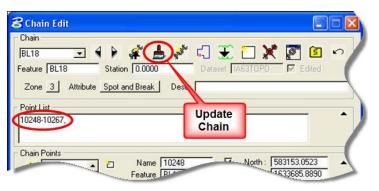
The modified BL survey chain is shown at the right. There is still a gap in the chain that must be repaired.
