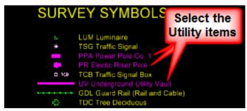
29.) Left-click the MicroStation Copy command, as shown at the right. Left-click once near the on the highlighted items to provide MicroStation with a "copyfrom" point. A copy of the highlighted items will now be attached to the cursor. Move the highlighted items to the correct position, similar to as shown below. Left-click to place the copy at that location. Right click to release the items from the cursor and then left-click on a blank area of the screen to un-highlight the items.
