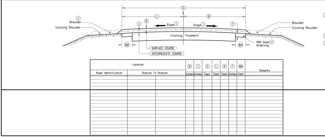
1 Match finished slope to existing pavement, except that the maximum allowable slope is 3.0%, minimum allowable slope is 2.0%. Section may be modified as directed by the Engineer through areas of special shaping.
