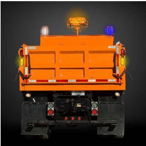
*Plow truck equipped with new white and blue rear facing lights as well as traditional amber light.*
