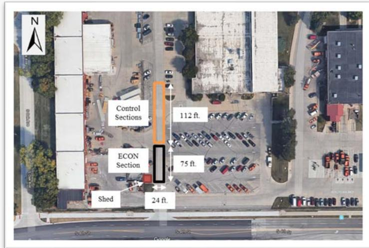
*Google earth image showing the project area. 4<sup>th</sup> Street is to the south at the bottom of the image. Note the project includes a control section of "regular" concrete immediately north of the electrically conductive section.*
