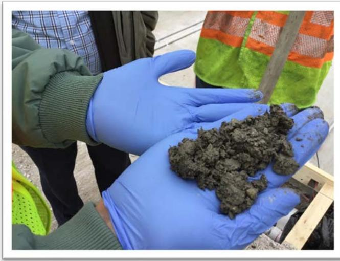
*The electrically conductive mix includes carbon fiber, which is an electrically conductive agent.*
