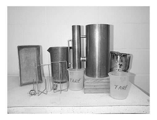
Figure 1. Volume-measuring Device
