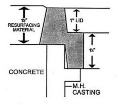
Vertically Adjustable. The riser used when lid thickness equals or exceeds the overlay thickness.
