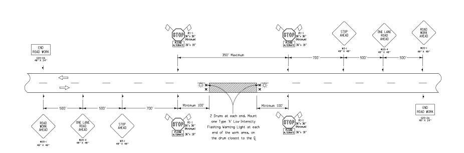
This layout shall not be used if the area between STOP signs is within a "No-Passing" zone.
