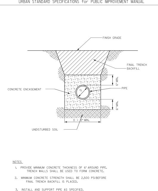
P.C. CONCRETE ENCASEMENT REV. DATE ΒY FIGURE: 3010.2 DATE: 01-01-98
