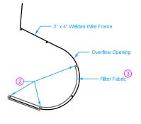
SEDIMENT FILTER CROSS SECTION
