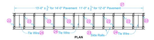
Spaces between dowel bars are nominal dimensions with a  $\frac{1}{4}$ " allowable tolerance.
