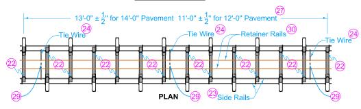
Spaces between dowel bars are nominal dimensions with a  $\frac{1}{4}$  allowable tolerance.
