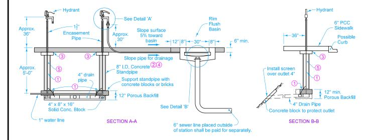
Install hydrants that are a combination freezeless and standard operating units or freezeless and self-closing (as designated on the plans), of a design and construction approved by the Engineer and equipped with approved model accessory attachment as indicated. Install riser pipe for hydrants that is one inch I.D. galvanized water pipe.
