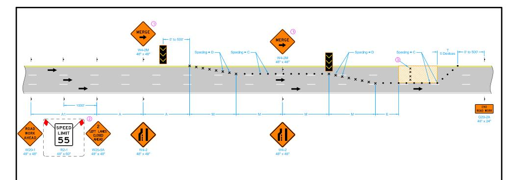
When the Average Daily Traffic (ADT) exceeds 20,000 vehicles per day or when a traffic queue extends beyond the advanced signing, place RIGHT/LEFT LANE CLOSED 4 MILES aigns (W20-5) on both sides of the roadway 4 miles and 2 miles in advance of the lane closure, respectively, as appropriate.
