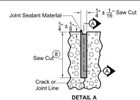
(Saw cut formed by conventional concrete sawing equipment.)
