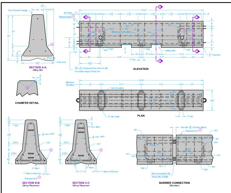
For loop bars 6d1, 6d2, and 6d3, use  $\frac{3}{4}$  smooth steel bars with a minimum yield strength of 60 ksi, a tensile strength of not less than 1.25 times the yield strength but a minimum of 80 ksi, a minimum 14% elongation in 8 inches, and passing a 180 degree bend test using a 3½" pin bend diameter.
