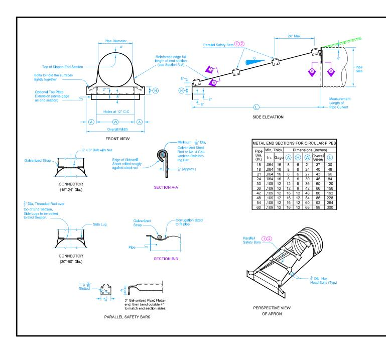
Install aprons and hardware fabricated from glavanized steel complying with Section 4141 of the Standard Specifications. Alternate design details may be submitted to the Engineer for approval
