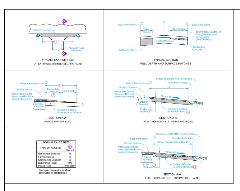
Unless specified otherwise, construct full runouts for HMA resurfacing at a rate of 50 feet for each 1 inch of resrufacing thickness.
